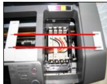
Rip the label on the balance arm
